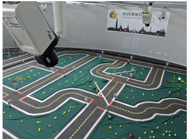
Figure 1: Cameras positioned above the model smart town enable participants to observe the situation from different angles. The smart town setup uses DuckieBot project-based roads and markers, that help DuckieBots navigate the road network.
